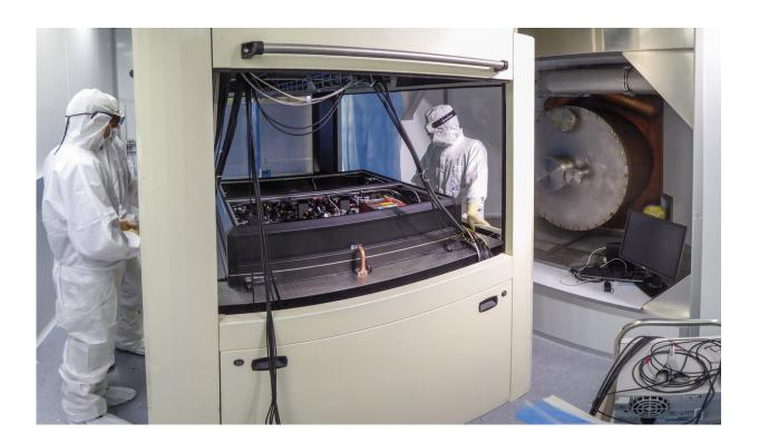
Together with their Virgo colleagues, the AEI researchers Harald Lück, Moritz Mehmet, and Henning Vahlbruch install the squeezed-light source, which was developed in Hannover, in a cleanroom at the Virgo gravitational-wave detector. Credit: H. Lück/B. Knispel/Max Planck Institute for Gravitational Physics
