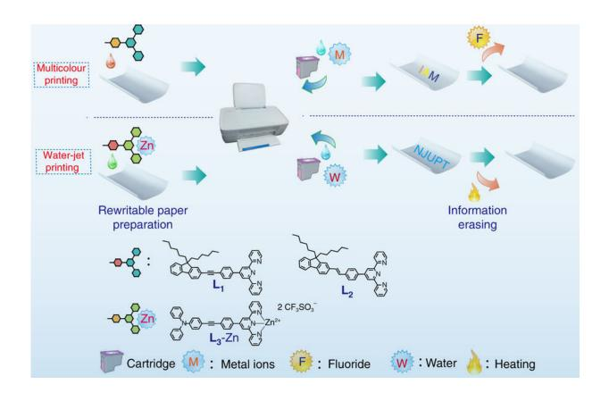
Schematic illustration of multicolour and water printing. Chemical structures of L 1 , L 2 and L 3 , and the printing and erasing processes for the constructed rewritable paper. Credit: *Nature Communications* (2017). DOI: 10.1038/s41467-017-02452-w
