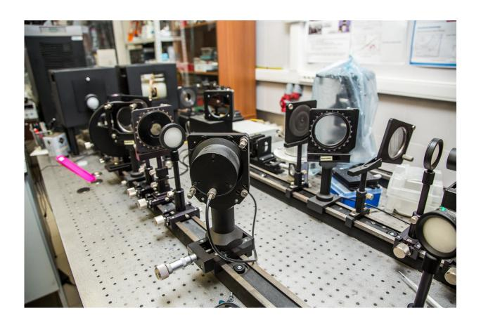
Some of the experimental data were obtained using a terahertz spectrometer based on backward-wave oscillators. Credit: MIPT
