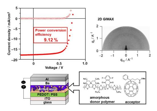
Fig.1.Current density-voltage characteristics of organic solar cell and X-ray pattern of active layer. Credit: Osaka University
