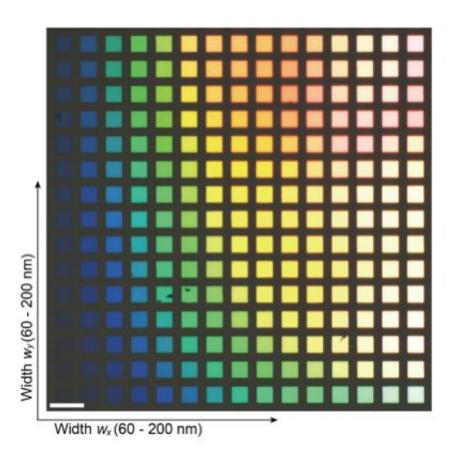
Fig.1. Bright-field optical microscope image of the Si nanostructure arrays. Si nanostructures of different sizes exhibit distinct reflection colors. (scale bar is 20  $\mu$ m). Credit: Takahara et al. *Nano Letters*. 17, 7500-7506. DOI: 10.1021/acs.nano-lett.7b03421
