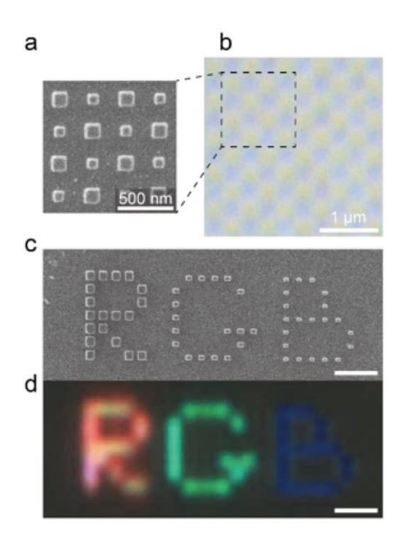
Fig.2. Demonstration of a subwavelength pixel. (a) Scanning ion and (b) optical microscope images of a checkered pattern consisting of alternating nanoblocks of two different sizes. (c) Scanning ion and (d) optical microscope images of the
