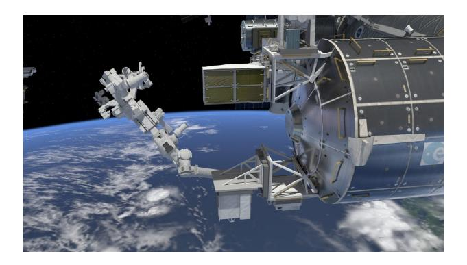
Mounted on the exterior of the International Space Station, the Space Debris Sensor (SDS) collects information on small orbital debris. Credit: NASA
