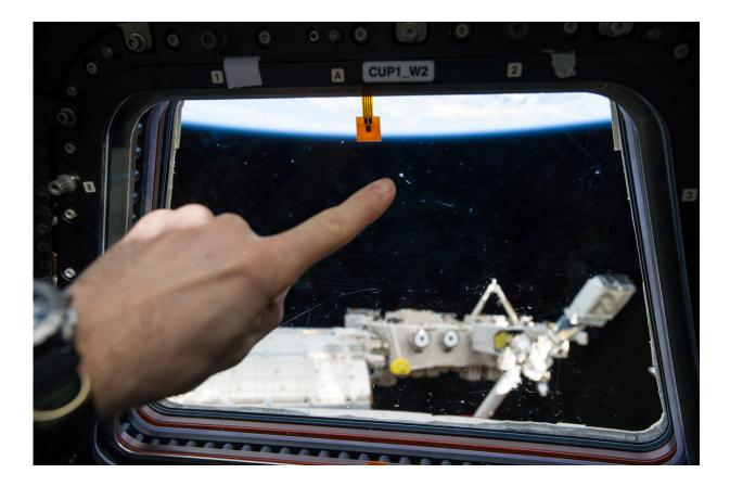
Photographic documentation of a Micro Meteor Orbital Debris strike one of the window's within the space station's Cupola. The Space Debris Sensor will measure the orbital debris environment for 2-3 years to provide impact detection and recording. Credit: NASA
