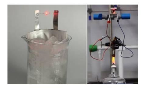
The battery works well in extreme tempratures. (Left: -30°C. Right: 100°C). Credit: Zhejiang University
