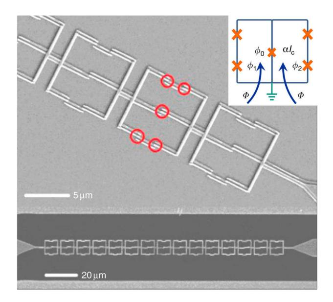
Superconducting quantum metamaterial consisting of an array of 15 twin qubits embedded in a coplanar wave guide. An SEM image of twin flux qubits (above)
