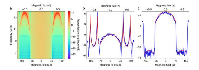
a The measured dependence of the amplitude of transmission coefficient t (normalized to the value at zero field) on applied dc magnetic field (proportional
