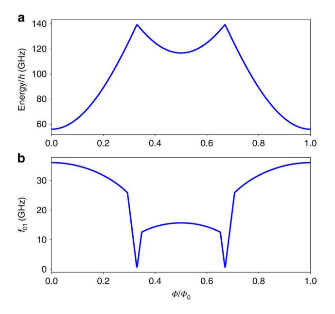
The energy of the ground state (a) and the transition energy hf01 of the twin qubit calculated from the Hamiltonian of Eq. (1) (b). The parameters  $\alpha$ ?=?0.72 and C?=?5.2 fF and the Josephson energy is E J ?=?50?GHz. These dependencies are  $\Phi$ 0 periodic and symmetric with respect to  $\Phi/\Phi$ 0?=?0.5. The minimum point of the (b) plot corresponds to the transition of the central junction phase  $\varphi$ 0 from zero to  $\pi$ . Credit: NUST MISIS
