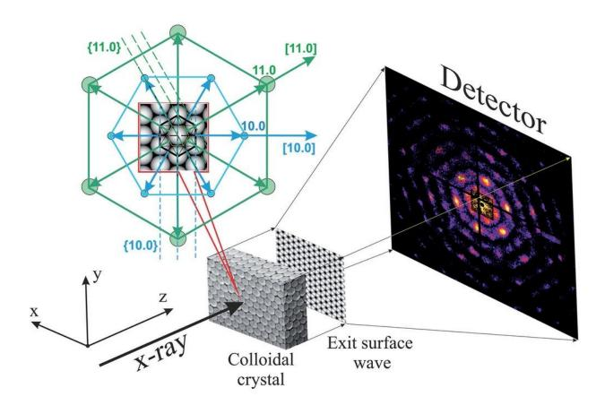
The scheme of analysis of photonic crystals' inner structure with the help of ptychography. Credit: ©NUST MISIS
