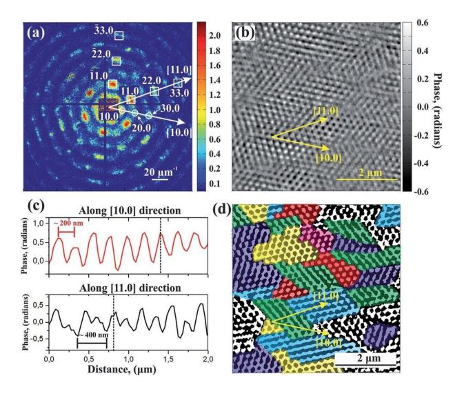
Photonic crystal received with the help of the method of ptychography. Credit: ©NUST MISIS
