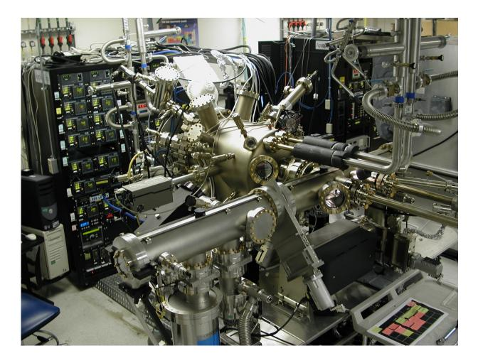
The Molecular Beam Epitaxy (MBE) is being used by Army researchers to produce new infrared detector materials based on InAsSb. This is a III-V semiconductor, a class of materials also used in opto-electronics in many commercial products such as DVD players and cell phones. Credit: US Army
