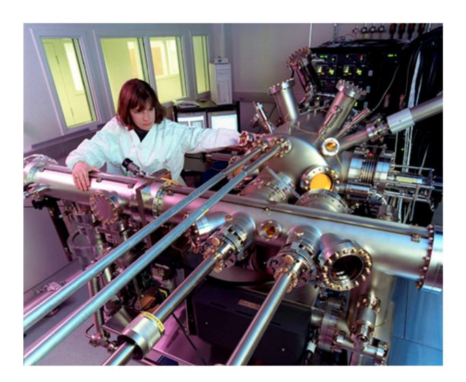
Dr. Wendy Sarney uses the molecular beam epitaxy machine at the US Army Research Laboratory to produce infrared detector materials with a new synthesis process. Credit: US Army
