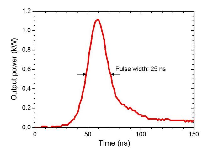
Obtained optical pulse. The peak power was about 1 kW. The pulse width was 25 ns. Credit: (c) Toyohashi University Of Technology.
