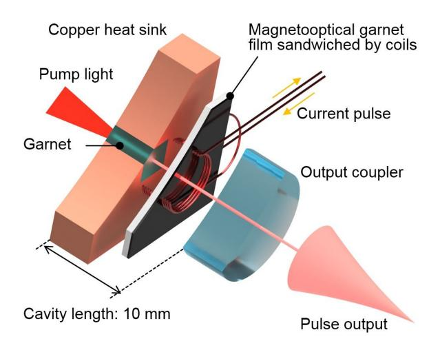
The first high-powered, randomly polarized laser beam with a 'Q switch' laser. Optical pulses were controlled by electrical signals. Credit: (c) Toyohashi University Of Technology.
