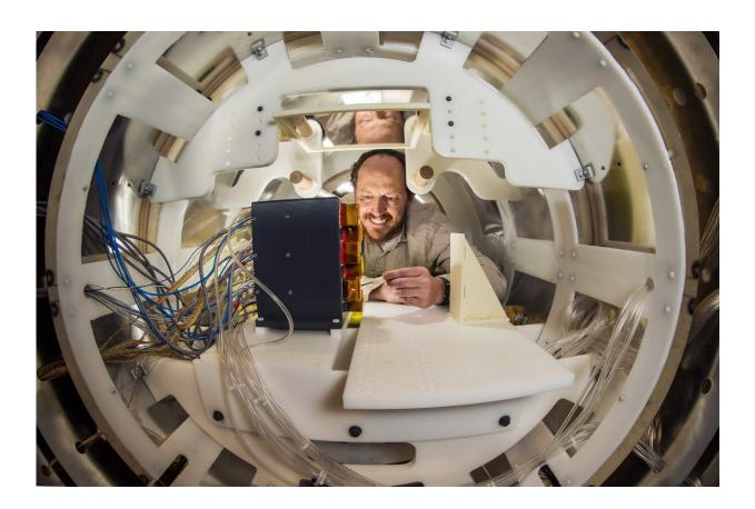
Peter Schwindt, Sandia National Laboratories principal investigator for a project to develop room-temperature magnetic sensors for magnetoencephalography, peers at an optically pumped magnetometer sensor array housed inside a personsize magnetic shield that resembles an MRI tube. Credit: Randy Montoya
