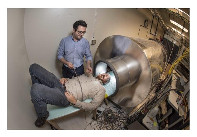
Sandia National Laboratories postdoctoral appointee Amir Borna, left, aids principal investigator Peter Schwindt in entering a person-size magnetic shield in preparation for a magnetoencephalography measurement with their optically pumped magnetometer array. Credit: Randy Montoya
