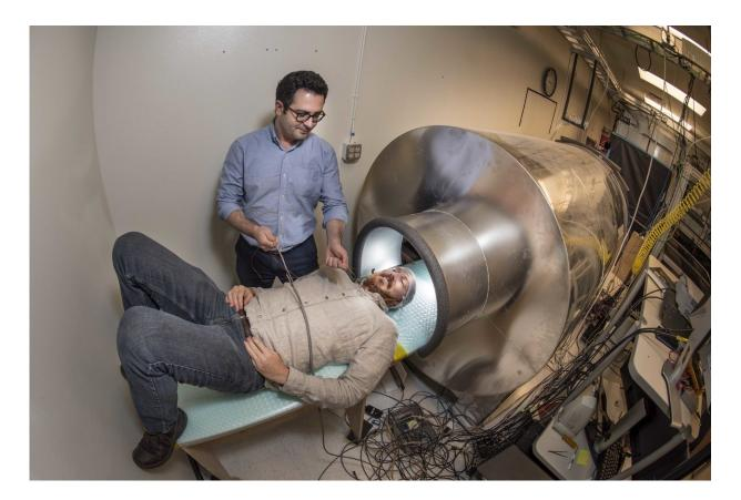
Sandia National Laboratories postdoctoral appointee Amir Borna, left, aids principal investigator Peter Schwindt in entering a person-size magnetic shield in preparation for a magnetoencephalography measurement with their optically pumped magnetometer array. Credit: Randy Montoya
