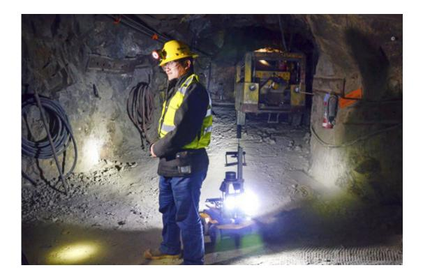
A miner is backed by a robot in the Edgar Mine near Denver, Colo., Dec. 13, 2017. The U.S. Environmental Protection Agency is considering robots and other technologies to investigate abandoned or inactive mines to learn what needs to be done with contaminated water spilling out of the mines and into rivers. Many of the mines are poorly understood and dangerous because of bad air and cave-ins. (AP Photo/Tatiana Flowers)
