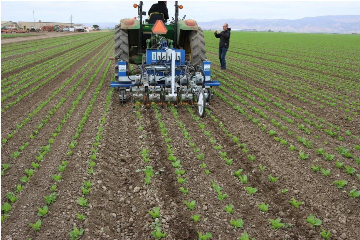
The robotic weeder goes between the crop rows. The rows must be very straight and precise for the weeder to properly do its job. Credit: Steven Fennimore
