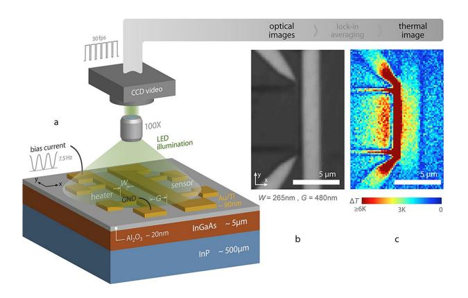
Purdue University researchers have visualized temperature changes produced by ultra-small heat sources, gold strips formed on top of the semiconductor indium gallium arsenide. The work has potential implications for the design of highspeed transistors and lasers. This image (a) depicts the device structure and experimental setup, an optical image (b) of the fabricated device and (c) an experimental thermal image. Credit: Purdue University image/Amirkoushyar Ziabari, Bjorn Vermeersch
