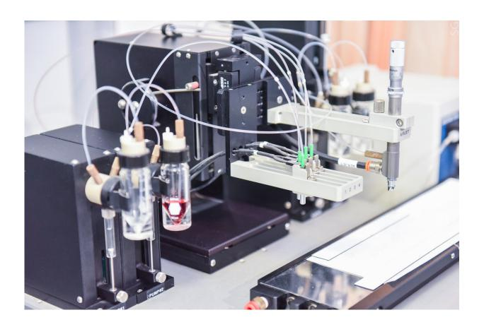
High-precision automatic dispenser for precise application of specific reagents. Credit: ©NUST MISIS
