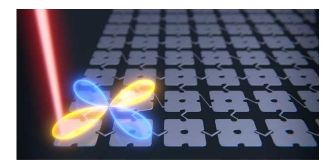
When the silicon wafer is stimulated at a single point using ultrasound, it begins to vibrate – but only at the corners. Credit: ETH Zürich
