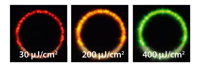
The quantum dot ring laser emits different colors of light at different laser powers. Credit: le Feber et al. ©2018 American Chemical Society
