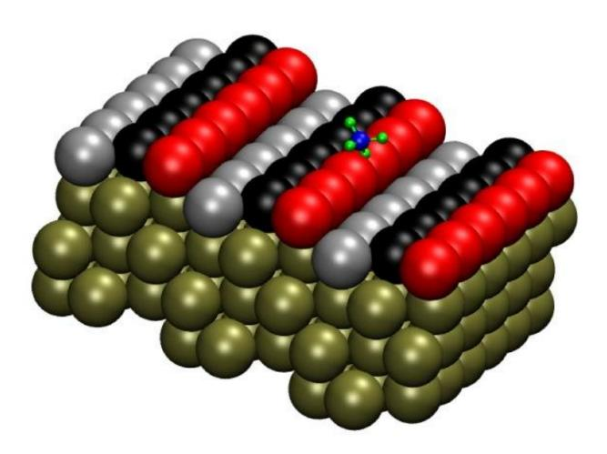
The Pt(211) surface has three-atom-wide terraces and one-atom-high steps. The researchers labeled the row of atoms on the step edge as "step" (red), the middle row as "terrace" (black) and the final row as "corner" (gray). Credit: Han Guo
