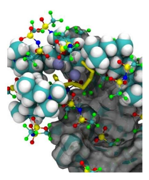
This illustration shows the formation of complex ion clusters during the cycling of a lithium-sulfur battery cell. The clusters consist of cationic polymer binders, battery electrolyte, and anionic sulfur-active materials. Credit: Berkeley Lab
