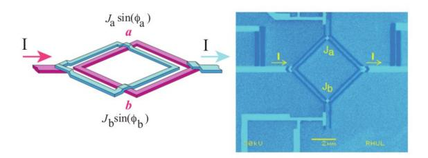
The schematic on the left shows two superconducting loops coupled by two Josephson junctions. The currents flowing through the Josephson junctions a and b are represented by Ja  $\sin(\varphi a)$  and Jb  $\sin(\varphi b)$ , respectively, where  $\varphi$  is the phase of the wave function — a quantum value characterizing the system as a whole. To the right is a false color image of the experimental system. Image courtesy of the authors of the research. Credit: 10.1021/acs.nanolett.7b01602
