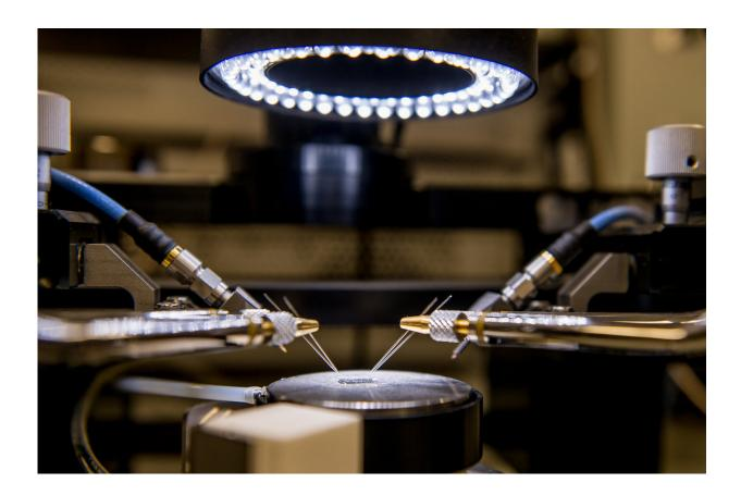
Electrophysical characteristics of the detector were tested on a probe station. Credit: Evgeniy Pelevin/MIPT
