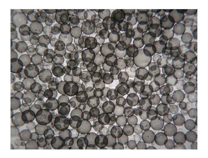
Micrograph of the graphene, water and oil emulsion developed by Uni of Sussex physicists. Credit: University of Sussex
