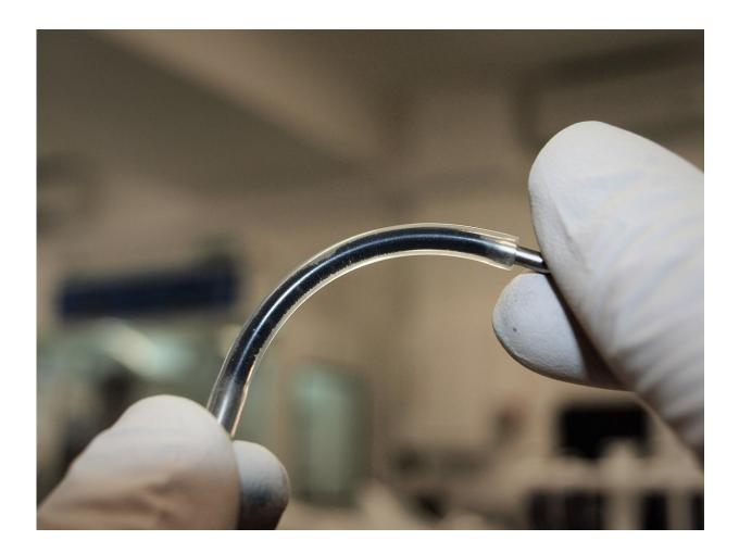
Sensing element of a prototype of the monitor device (flexible pipe filled with graphene emulsion) -- developed by University of Sussex physicists. Credit: University of Sussex
