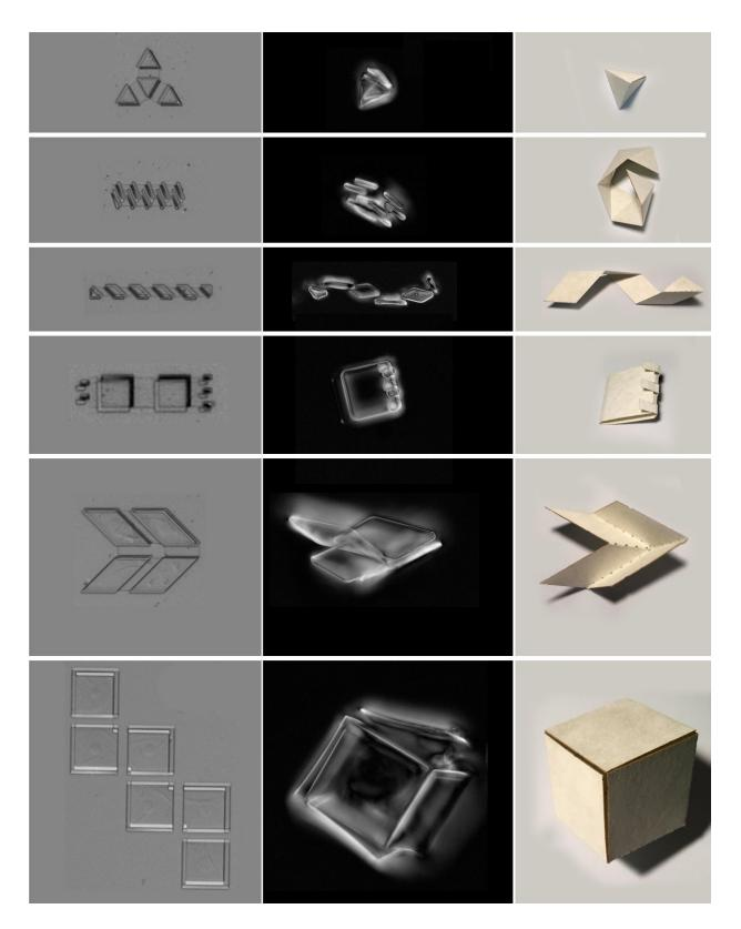
Graphene-glass bimorphs can be used to fabricate numerous micron-scale 3-D
