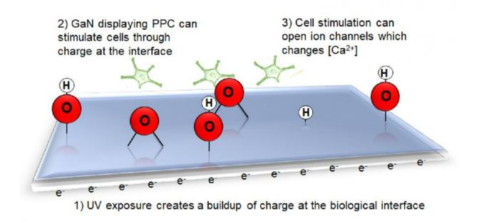
Exposure of GaN to UV light causes an accumulation of electrons at the biological interface even after the light is removed. This phenomenon, known as persistent photoconductivity (PPC), can be used to stimulate neurotypic cells in a way that can modulate the amount of calcium in cells. Credit: North Carolina State University
