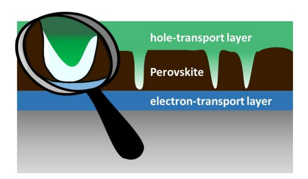
Simplified cross-section of a perovskite solar cell: the perovskite layer does not cover the entire surface, but instead exhibits holes. The scientists could show that a protective layer is being built up which prevents short circuits. Credit: HZB
