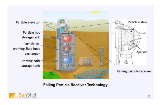
Particle receiver diagram. Credit: Sandia
