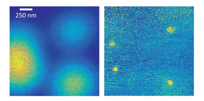
Whereas the image taken with a normal microscope is blurry (left), the new method (right) clearly shows four quantum dots (bright yellow spots). Credit: University of Basel, Department of Physics
