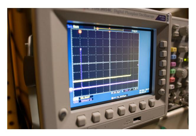
Pulses on the oscilloscope indicate when the particles arrive in the detector. Credit: Reidar Hahn
