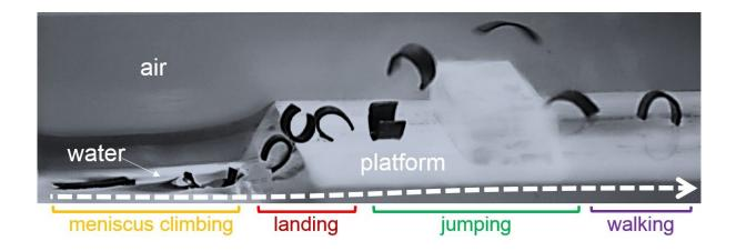
The soft millirobot climbs on the water meniscus by changing its body curvature and lands on the solid surface. Next, it encounters a large obstacle and traverses it fast and easily by jumping over it, and walks on the surface after landing. The dashed line shows the direction of the robot motion. Credit: Max Planck Institute for Intelligent Systems
