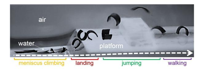
The soft millirobot climbs on the water meniscus by changing its body curvature and lands on the solid surface. Next, it encounters a large obstacle and traverses it fast and easily by jumping over it, and walks on the surface after landing. The dashed line shows the direction of the robot motion. Credit: Max Planck Institute for Intelligent Systems
