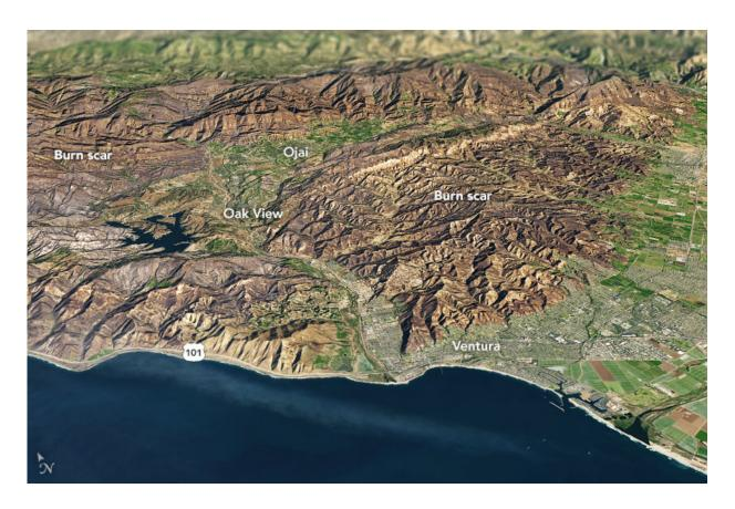
The Operational Land Imager (OLI) on Landsat 8 captured an image of the Thomas fire scar in California on Dec. 18, 2017. The natural-color Landsat 8 image was draped over an ASTER-derived Global Digital Elevation Model, which shows the topography of the area. Credit: NASA Earth Observatory, Joshua Stevens; USGS; NASA/GSFC/METI/ERSDAC/JAROS, and U.S./Japan ASTER Science Team.
