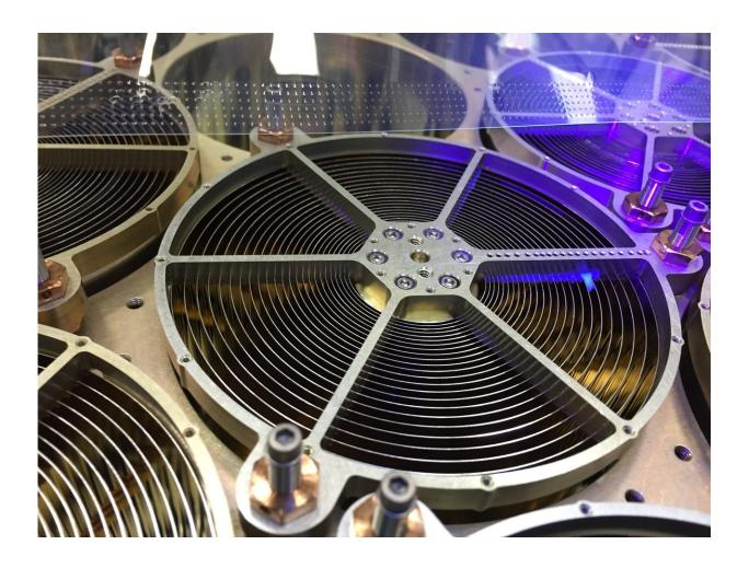
NICER's mirror assemblies concentrate X-rays onto silicon detectors to gather data that probes the interior makeup of neutron stars, including those that appear to flash regularly, called pulsars. Credit: NASA's Goddard Space Flight Center/Keith Gendreau
