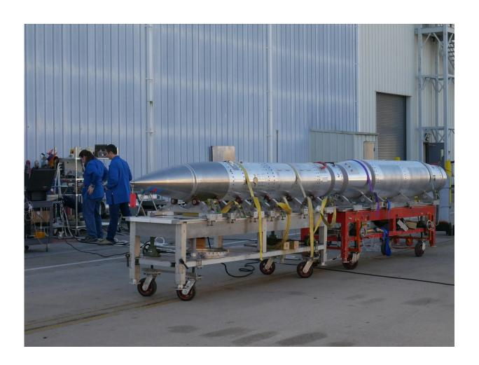
Personnel at the Wallops Flight Facility test the DXL payload's ability to connect with the Global Positioning Satellite (GPS) network which will be used to determine the location of the payload during flight. Credit: NASA/Berit Bland
