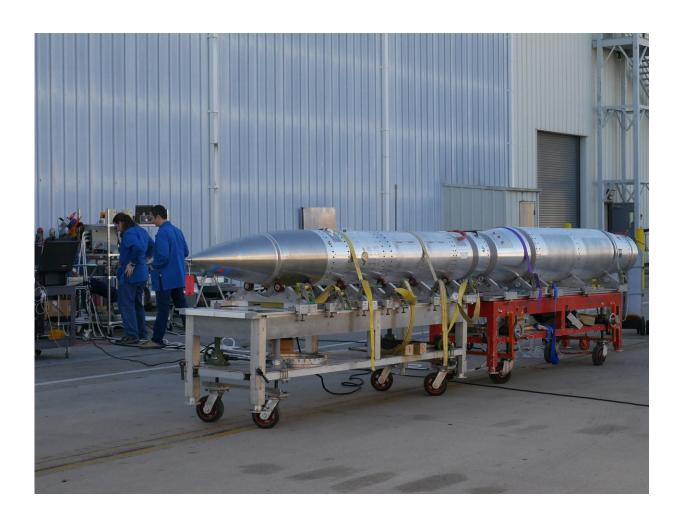
Personnel at the Wallops Flight Facility test the DXL payload's ability to connect with the Global Positioning Satellite (GPS) network which will be used to determine the location of the payload during flight. Credit: NASA/Berit Bland
