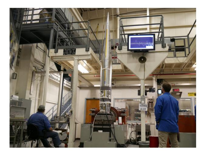
A Super Soaker payload is tested for its ability to operate while experiencing vibrations during flight. Credit: NASA/Berit Bland
