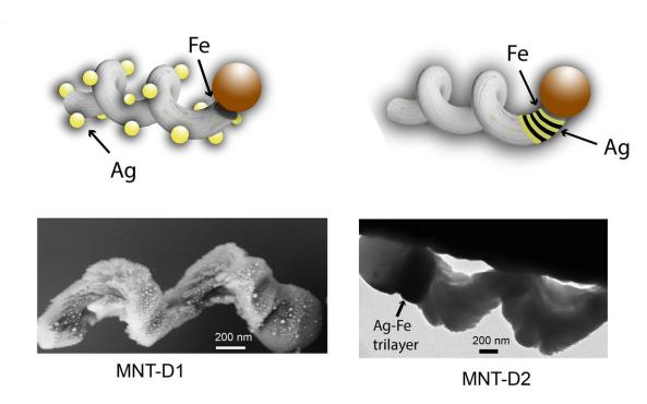
The mobile nanotweezers are comprised of a screw-shaped magnetic microrobotic body dotted with silver particles that cluster in response to light. Credit: Ghosh and Ghosh, *Sci. Robot.* 3, eaaq0076 (2018)
