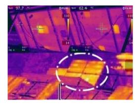
An infrared photo shows how reflectors send more light toward solar panels to produce more power. Credit: Joshua M. Pearce, CC BY-SA
