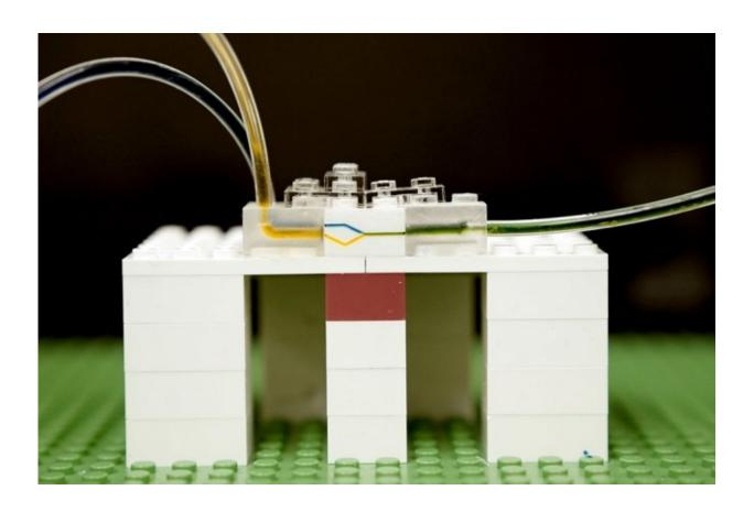
MIT researchers have developed a new platform for microfluidics, using LEGO bricks. Shown here, fluid flows through tiny channels milled into the side walls of LEGO bricks. Credit: Massachusetts Institute of Technology
