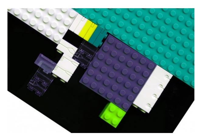
A close-up of LEGO bricks, milled with tiny fluidic channels. Credit: Massachusetts Institute of Technology
