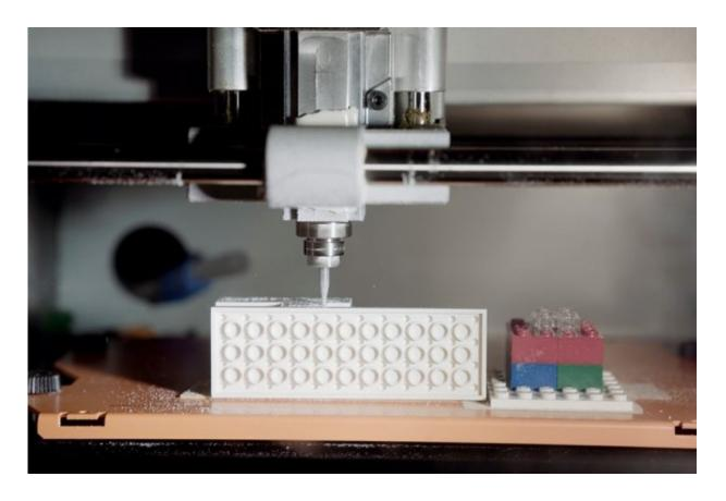
MIT researchers used a desktop micromilling machine to drill small channels into the sidewalls of LEGO bricks. Credit: Massachusetts Institute of Technology
