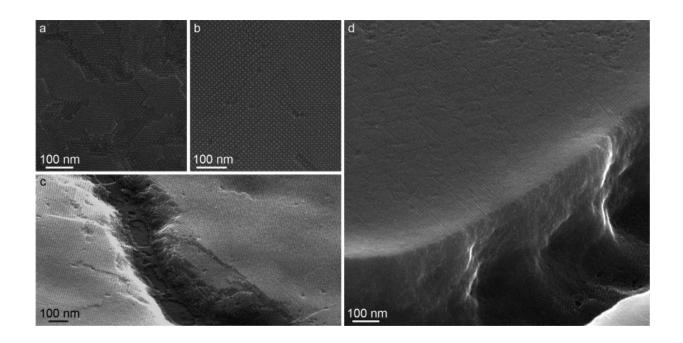
These images show scanning electron micrographs of the researchers' sample quantum dot films. The dark spots are the individual quantum dots, each about 5 nanometers in diameter. Images a and b show the consistent size and alignment of the quantum dots at the surface. The exposed edges in images c and d show depth and long-range ordering of the nanocrystals. Credit: Massachusetts Institute of Technology
