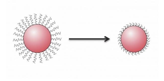
As shown in these schematics, at the center of a quantum dot is a core of a semiconducting material. Radiating outward from that core are arms, or ligands, of an organic material. The ligands keep the quantum dots in solution from sticking together, and they determine the spacing between the dots in the solid product. Replacing the long ligands on the left with the short ones on the right allows the quantum dots to pack more closely together. Credit: Massachusetts Institute of Technology
