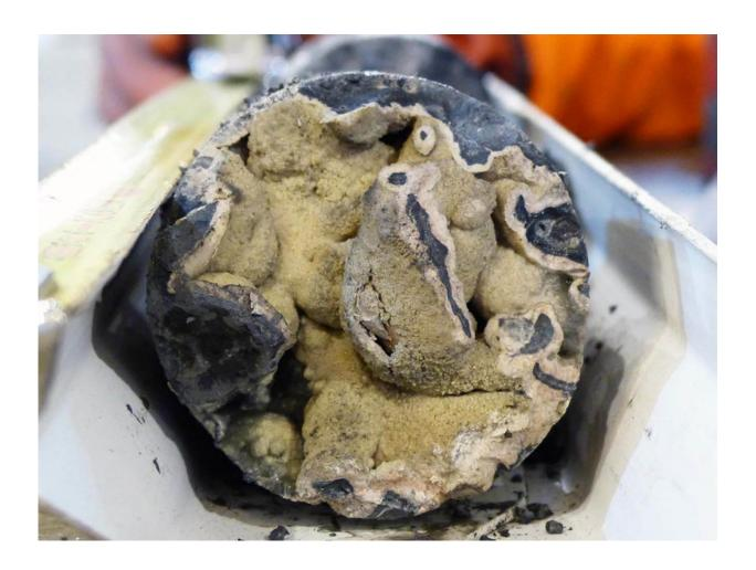
The rotary drill bit of the MeBo70 has penetrated a layer of limescale activated in soft sediments. Bright aragon cements typically fill the cavities of the sea carbonates. Credit: MARUM - Zentrum für Marine Umweltwissenschaften, Universität Bremen; G. Bohrmann
