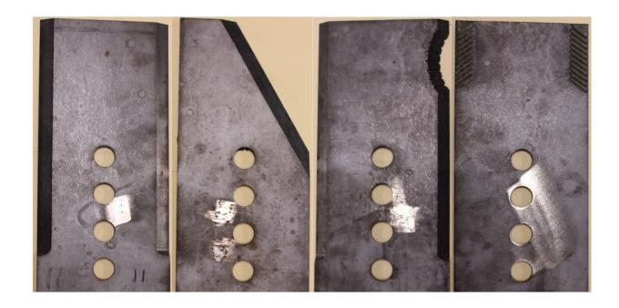
Four blades were tested to cut sugarcane. Left to right: straight, angled, serrated, and straight with laser clad underside. The serrated blade performed best. Credit: University of Illinois
