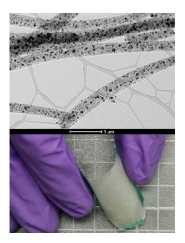
Engineered carbon fibers embedded with active nanoparticles (top) can be fabricated into structural materials that are lightweight and flexible (bottom). Credit: UC Riverside
