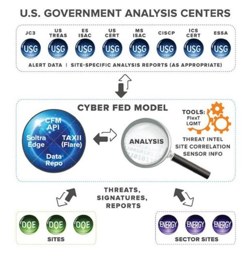
Argonne's Cyber Fed Model routes cyberthreat indicators in near real-time and provides defensive measures and tools to simplify use of this information. Once a participating local system spots an attack, it can be rapidly shared to enable local damage mitigation and prevent its spread. Credit: Argonne National Laboratory
