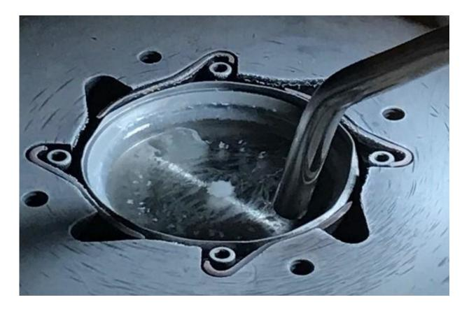
Closer look at the target of frozen solution that contains the building blocks for the solar cell material. Credit: E. Tomas Barraza
