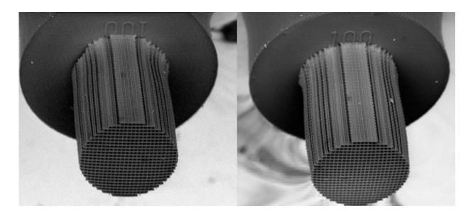
LLNL researchers printed octet truss structures with submicron features on top of a solid base with a diameter similar to human hair. Credit: James Oakdale/LLNL
