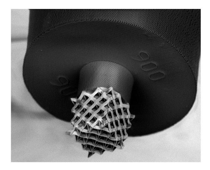
Through the two-photon lithography (TPL) 3D printing process, researchers can print woodpile lattices with submicron features a fraction of the width of a human hair. Credit: James Oakdale/LLNL
