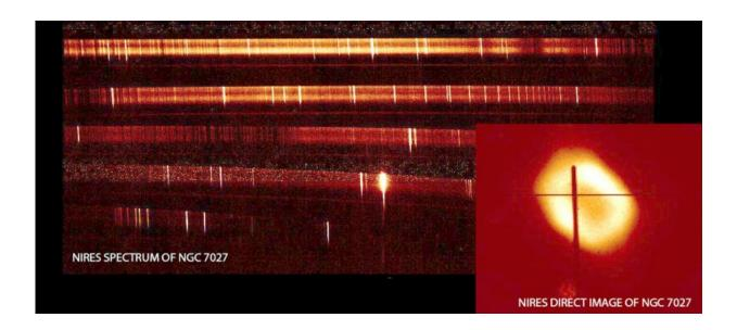
The "first-light" image from NIRES is of NGC 7027, a planetary nebula. The NIRES spectrum shows the near-IR spectrum of this nebula dominated by emission lines of hydrogen and helium. The direct image shows NBC 7027 in the K' filters at 2.2 microns. Credit: W. M. Keck Observatory
