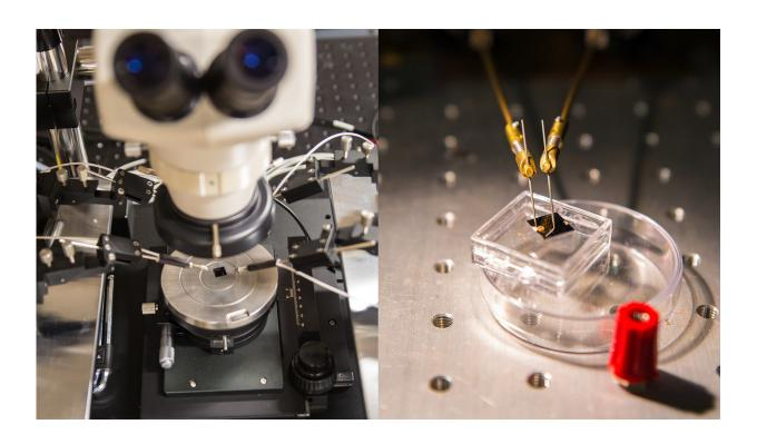
The probe-station device (the full instrument, left, and a closer view of the device connection, right) which measures the electrical responses of the basic components for computers mimicking the human brain. The tunnel junctions are on a thin film on the substrate plate. Credit: Tapio Reinekoski
