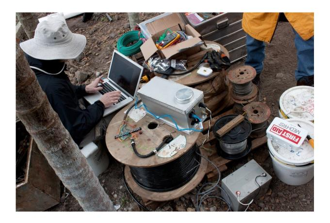
Scientists in Taiwan prepare to install several borehole strainmeters into the ground to monitor ground deformation after tropical cyclones pass overhead. Credit: Maxime Mouyen
