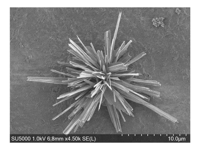
The surface of a nanostructured copper catalyst that converts CO2 into ethylene. Credit: Canadian Light Source
