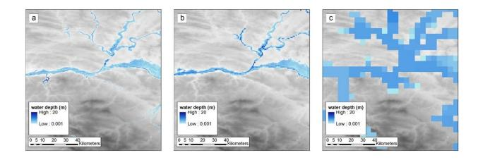
Inundation maps for a 1 in 100 year flood event along the Loire River (France) from three different inundation models. The resolution of flood models is a key component to improve flood risk assessments.
