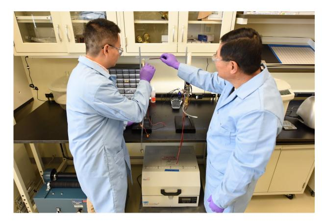
Research scientists Dong Ding (left) and Ting He developing direct carbon fuel cells at INL's Energy Innovation Laboratory. Credit: Idaho National Laboratory
