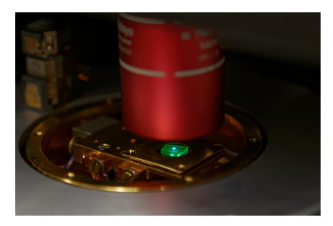
A sample with several green glowing perovskite quantum dots excited by a blue laser. Credit: IBM Research / Thilo Stoeferle
