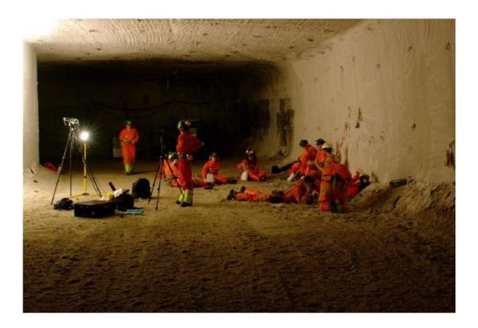
Testing of laser Raman spectroscopy prototype for ESA's ExoMars rover, taking place in Boulby salt mine in North Yorkshire, which has geological similarities to the surface of Mars, including chloride and sulphate deposits. Credit: Matthew Gunn
